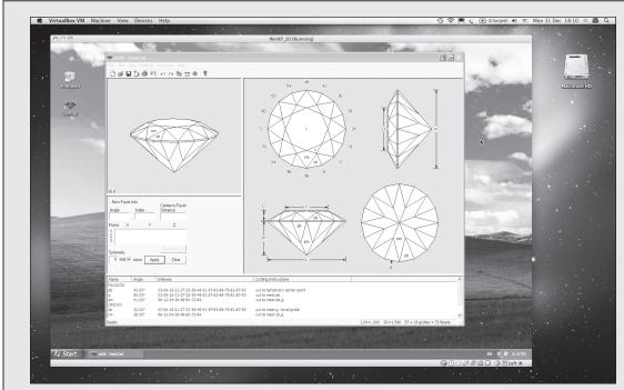
Figure 15-2 Virtualization tools such as VirtualBox let you run Windows programs, including GemCAD, under other operating systems. Look carefully at the screenshot – yes, that is indeed GemCAD running on a Windows XP virtual computer which is, in turn, running "inside" a Mac.
